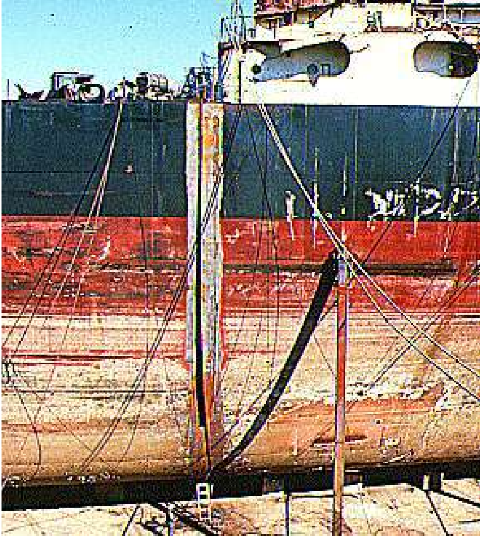
Figure 1: Bisecting a ship in order to install a new section (Encyclopedia of occupation health and safety 4 th Edition)
